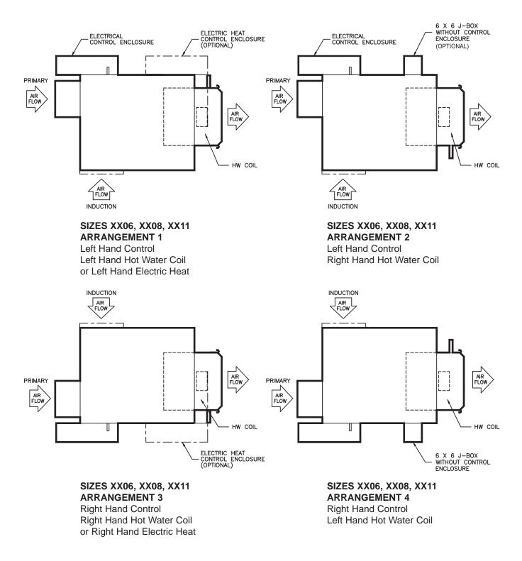
**NOTE:** Induction location shown is typical of unit sizes 06, 08 and 11 as shown on Dimensional Drawings. Size 19 induction inlets are located on both sides of the primary air inlet and are not influenced by handing arrangement.
